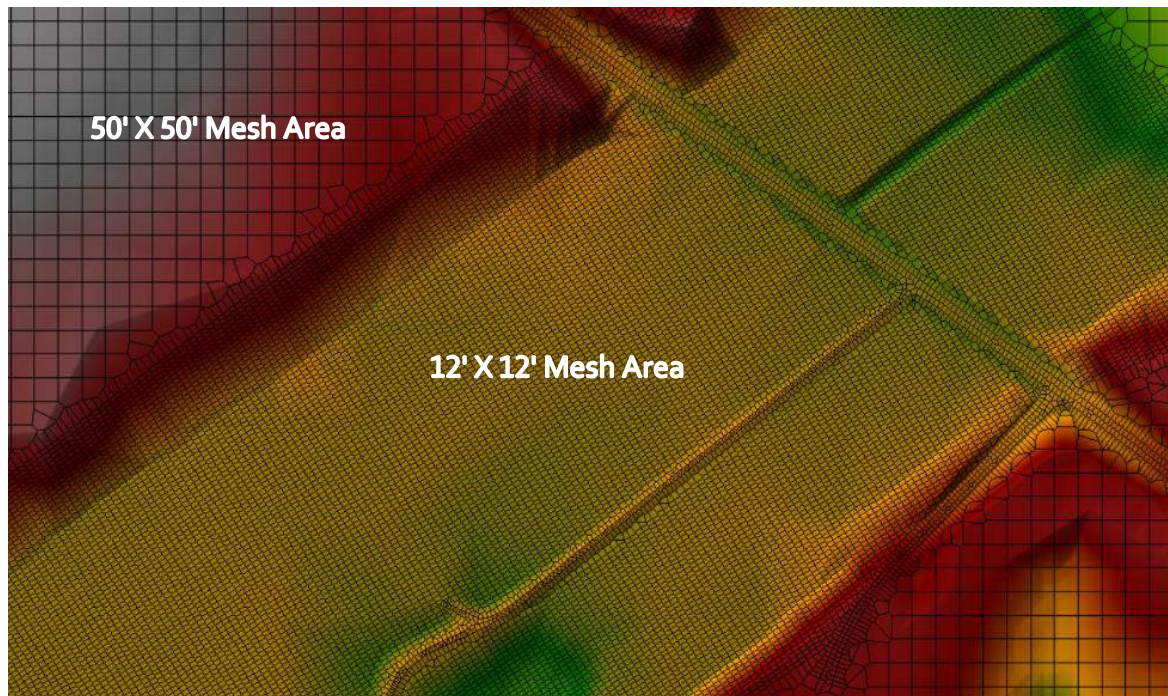
Figure 14: HEC-RAS 50x50 and 12x12 Mesh over a Portion of the Emergency Spillway and FM 3122
